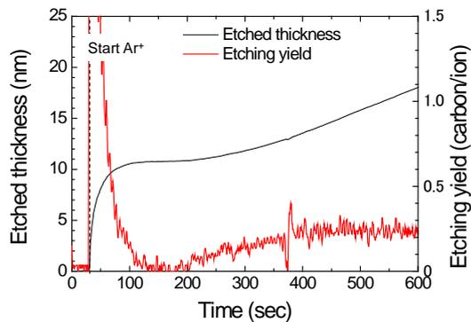
Fig. 6. Exposure time dependence of etched thickness and etching yield of photoresist
