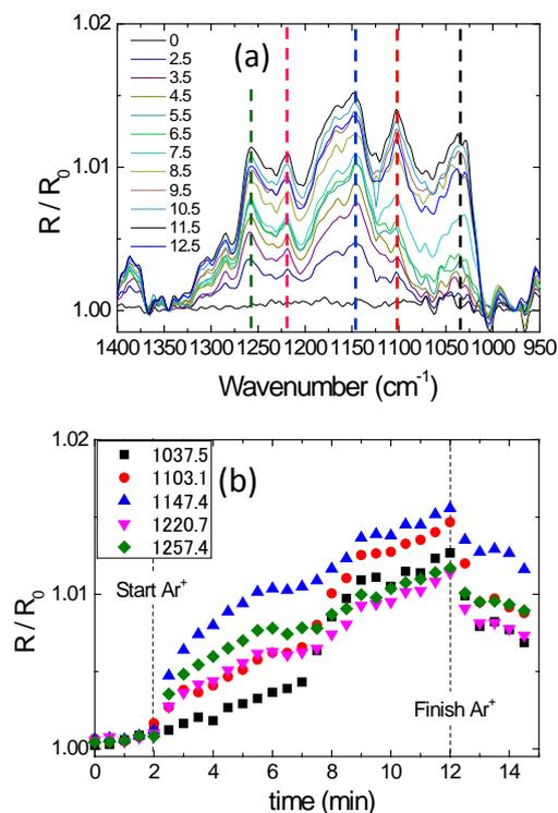
Fig. 5. Beam exposure time dependence of C-O
