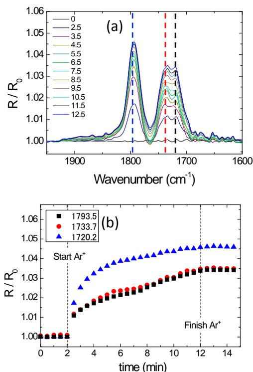
Fig. 4. Beam exposure time dependence of C=O
