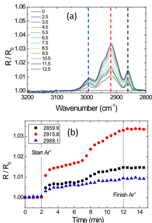
Fig. 3. Beam exposure time dependence of C-H<sub>x</sub> (a) Spectra of IR absorption (b) Peak height changes
