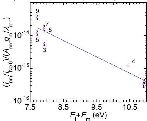
Fig.5. Emission intensity ratio plotted as a function of electron energy.
