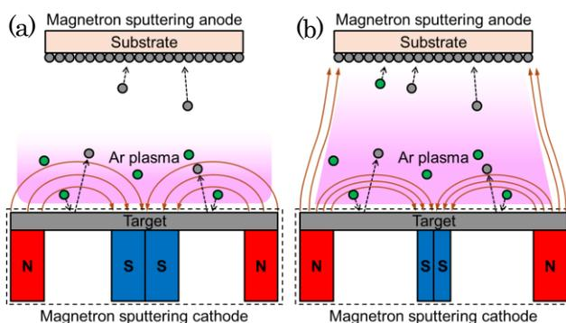
Fig. 1 (a) Conventional magnetron sputtering and (b) UBM sputtering
