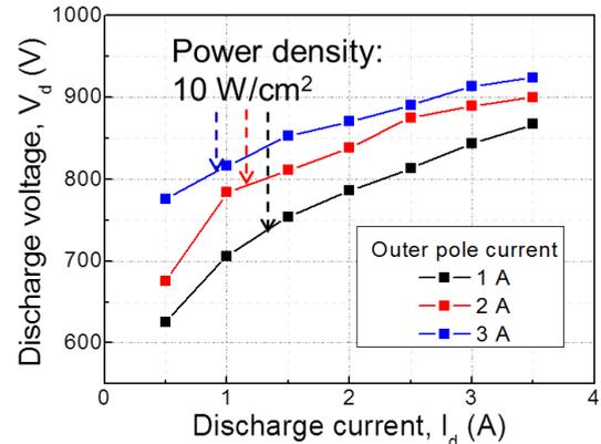
Fig. 4  $I_d$ - $V_d$  characteristics for each inner pole current
