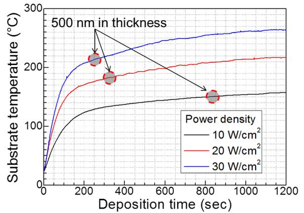
Fig. 6 Time dependence of substrate temperature
