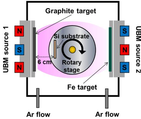
Fig. 2 CFUBM sputtering system [1]
